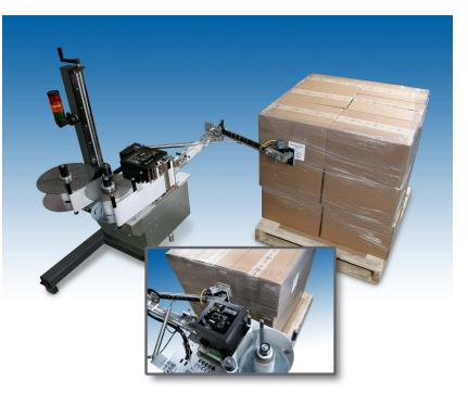
Weber's Model 5300 Dual-Label pallet printer-applicator marries a high-performance thermal/thermal-transfer label printer with a specially-engineered articulating swing-tamp applicator to perform the printing and two-label, adjacent-side labeling of pallets in line.
