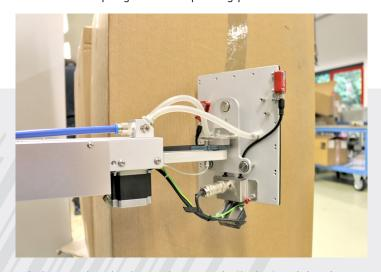
Labels are printed using an integrated printing module. The rectangular AP 182 printing dispenser system enclosure comprises a profiled frame construction with stainless steel cladding, except for the transparent side door. High AP 182 flexibility allows up to 7 different movement profiles, variably combinable per pallet. This allows individual 1-, 2- or 3-sided labelling of each approaching pallet.
